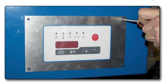
2. Delicately remove the plate from the front of the machine.
