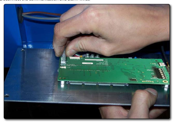
4. Be sure to identify the oil sensor wire before disconnecting.
