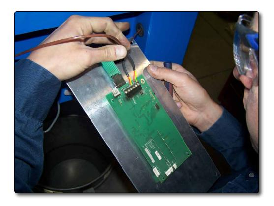
11. Re-connect the grey comm. wire and the red and black alarm wire. Take special care to properly align the wires when installing.
